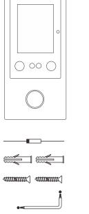
Diode IN4004 (For relay circuit protection)
