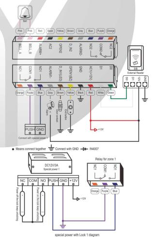
Mode Standalone for single door diagram DC12V special power
